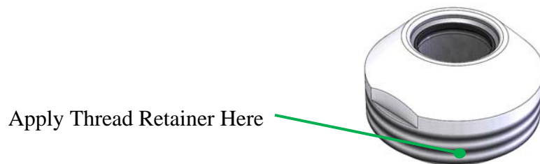
Figure 52: Thread Retainer Location on Nozzle
