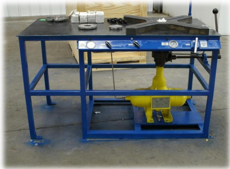
Figure 1: ENG-511001 Mercer Valve's Test Stand
