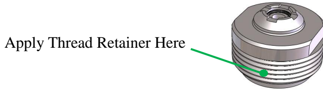
Figure 25: Thread Retainer Location on Nozzle
